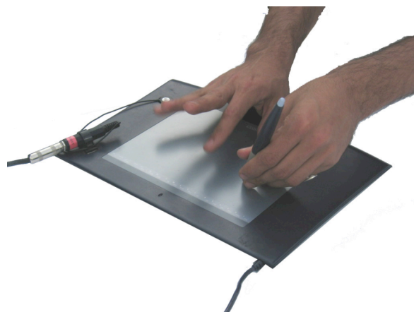
Figure 3. Mixed sensing of the tablet by way of audio input from a contact microphone placed on the tablet’s body. The performer plays the tablet like a percussion instrument with one hand while he manipulates the pen with the other hand in order to modulate synthesized sounds.
